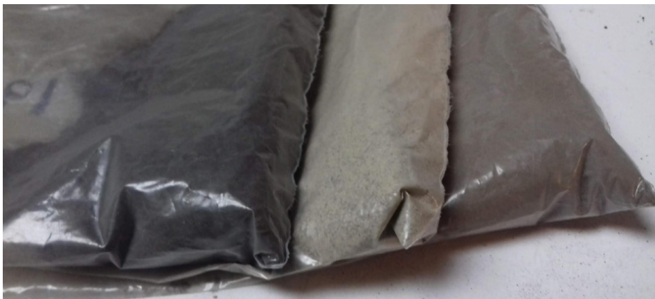
Figure 2. Dried, ground, and sifted compounded soil samples in labeled airtight plastic bags. Here we see three samples at three different depths of the same site.
