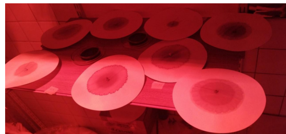
Figure 3. Running diluted soil samples on paper previously impregnated with \text{AgNO}_3 .
