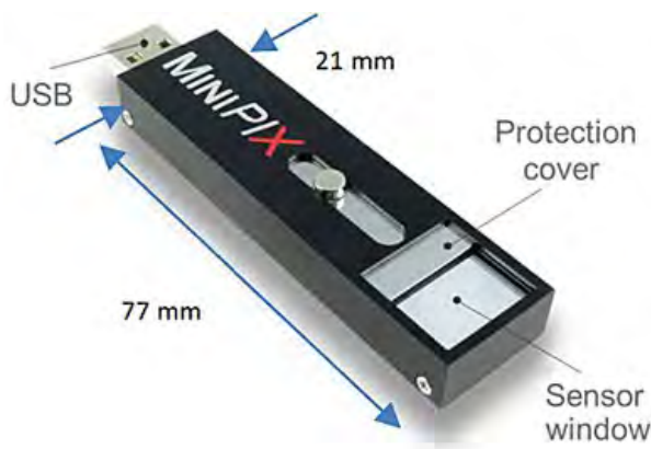
Figure 2. Miniaturized radiation camera MiniPIX-Timepix. Size dimensions 77 mm × 21 mm × 10 mm and connects directly to PC or laptop via single USB connector [5].
