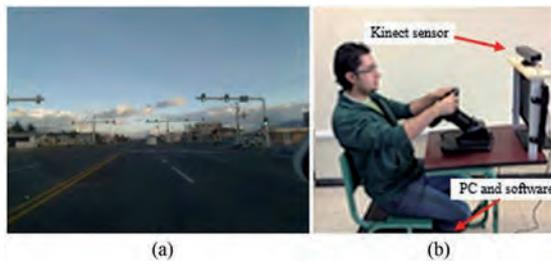
Figure 1: Driving simulator: (a) scene from a video of an Ecuadorian road, (b) Kinect hardware and the software developed in this research.
