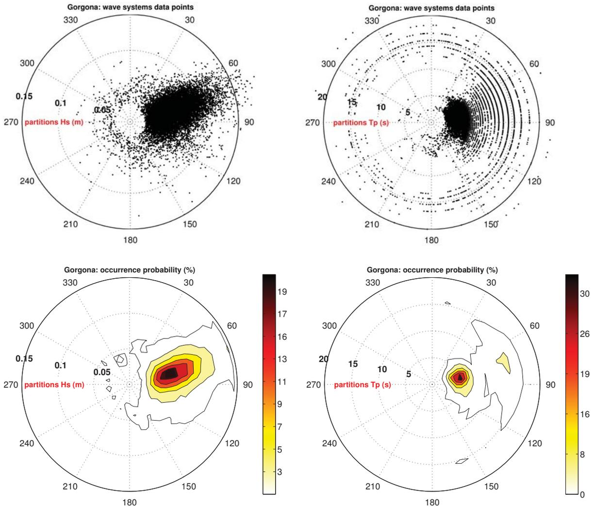
Figure 6: Statistics of  $H_{m0}$  (left) and  $T_{m-1,0}$  (right) for wave spectral partitions at Gorgona.
