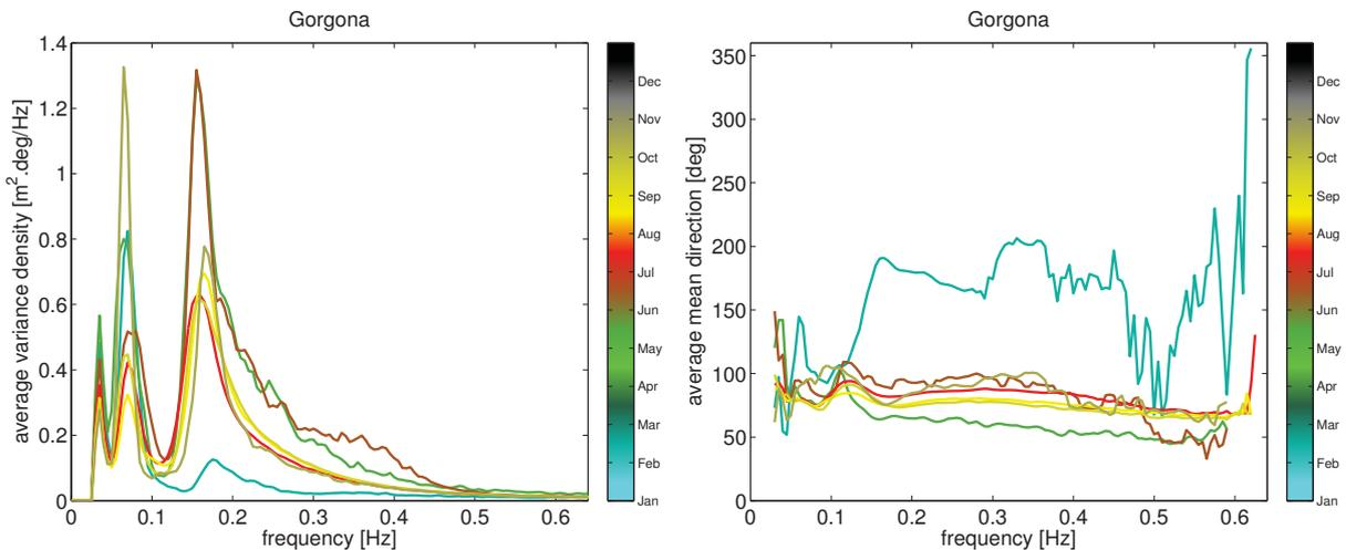
Figure 10: Monthly statistics of the frequency spectrum: variance density (left), and mean direction (right) at Gorgona.
