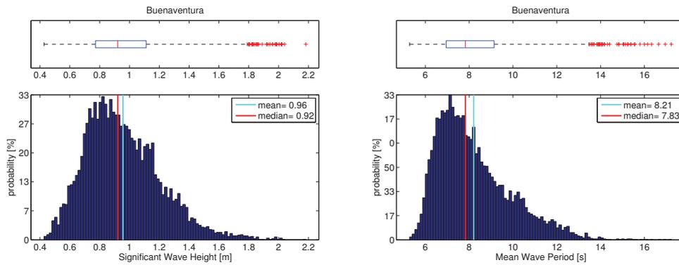
Figure 15: Statistics of integral parameters over the whole spectrum,  $H_{m0}$  (left) and  $T_{m-1,0}$  (right) at Buenaventura.
