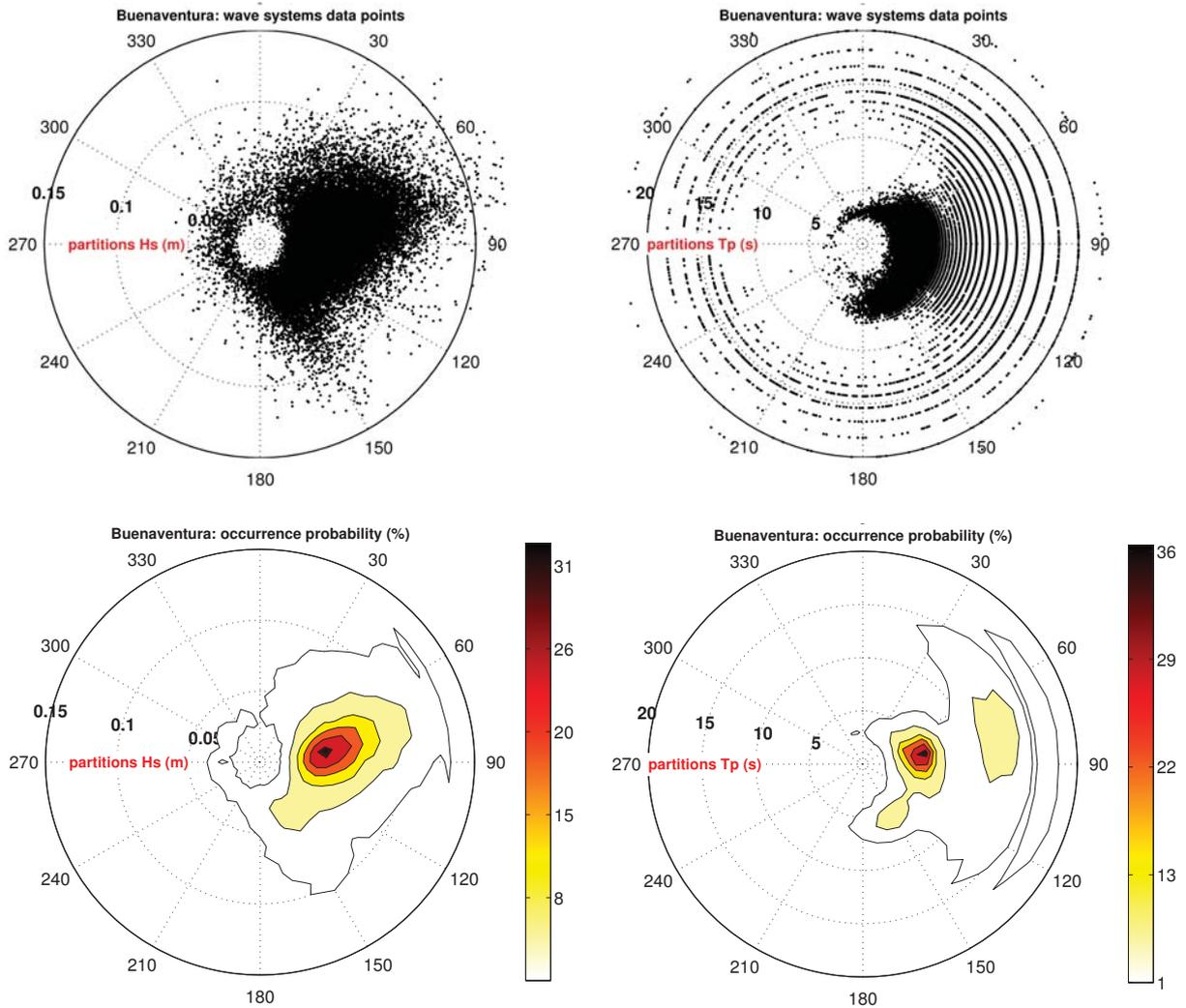
Figure 7: Statistics of  $H_{m,0}$  (left) and  $T_{m-1,0}$  (right) for wave spectral partitions at Buenaventura.
