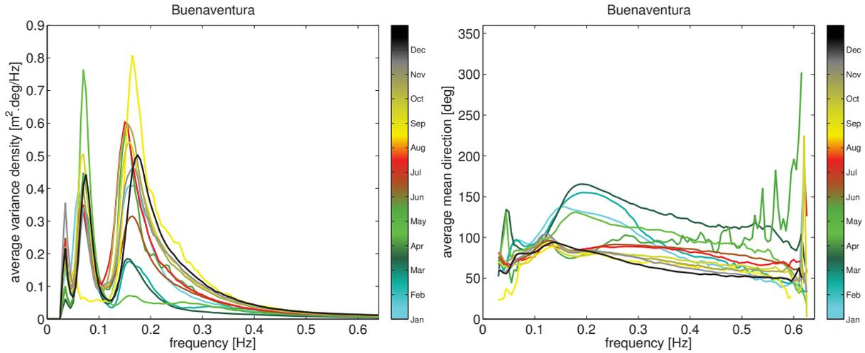
Figure 11: Monthly statistics of the frequency spectrum: variance density (left), and mean direction (right) at Buenaventura.
