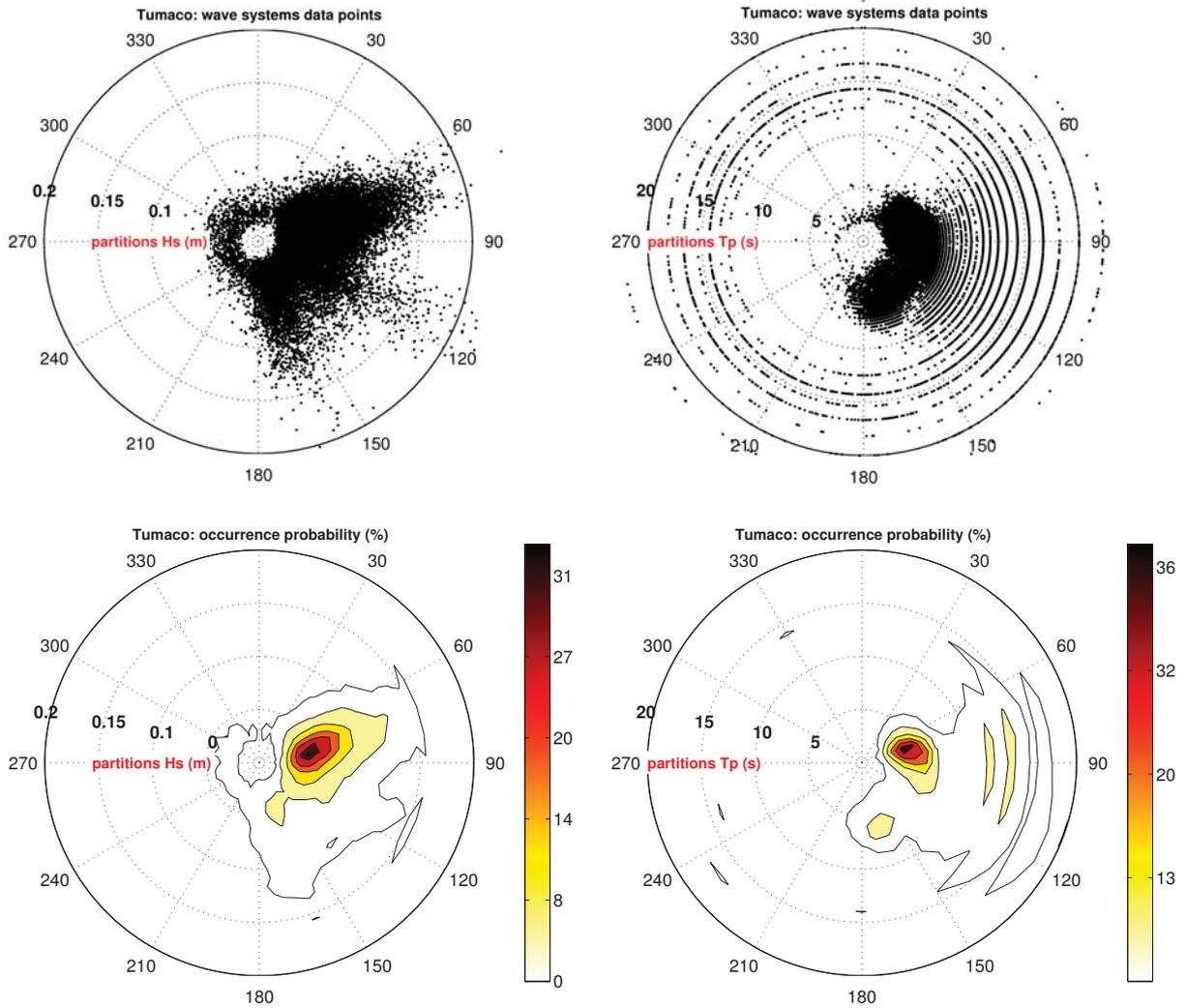
Figure 5: Statistics of  $H_{m0}$  (left) and  $T_{m-1,0}$  (right) for wave spectral partitions at Tumaco.
