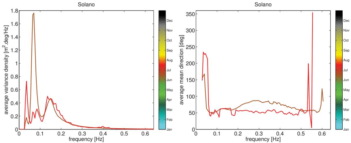
Figure 12: Monthly statistics of the frequency spectrum: variance density (left), and mean direction (right) at Solano.
