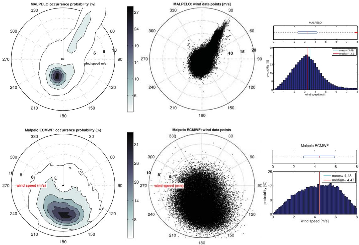
Figure 4: Wind statistics from observed records (upper panels), and from the ECMWF model (lower panels) at Malpelo.
