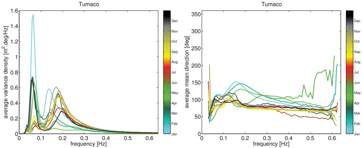
Figure 9: Monthly statistics of the frequency spectrum: variance density (left), and mean direction (right) at Tumaco.
