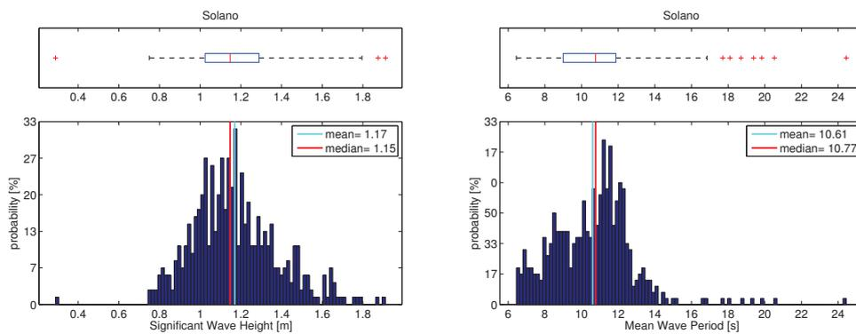
Figure 16: Statistics of integral parameters over the whole spectrum,  $H_{m0}$  (left) and  $T_{m-1,0}$  (right) at Solano.
