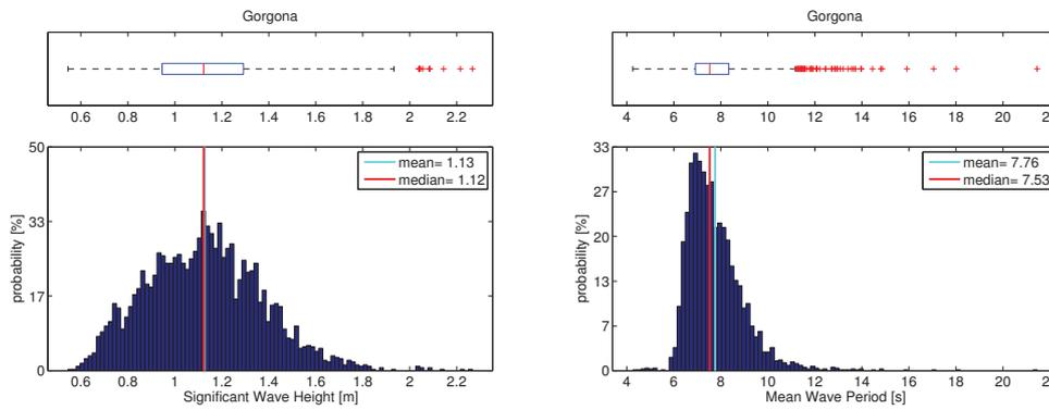
Figure 14: Statistics of integral parameters over the whole spectrum,  $H_{m0}$  (left) and  $T_{m-1,0}$  (right) at Gorgona.
