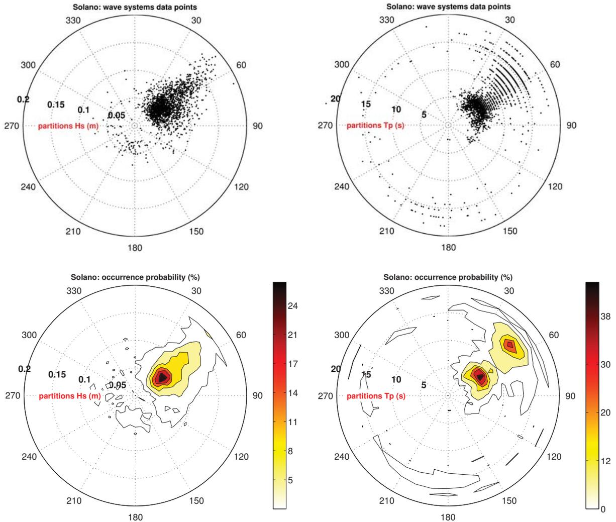
Figure 8: Statistics of  $H_{m0}$  (left) and  $T_{m-1,0}$  (right) for wave spectral partitions at Solano.
