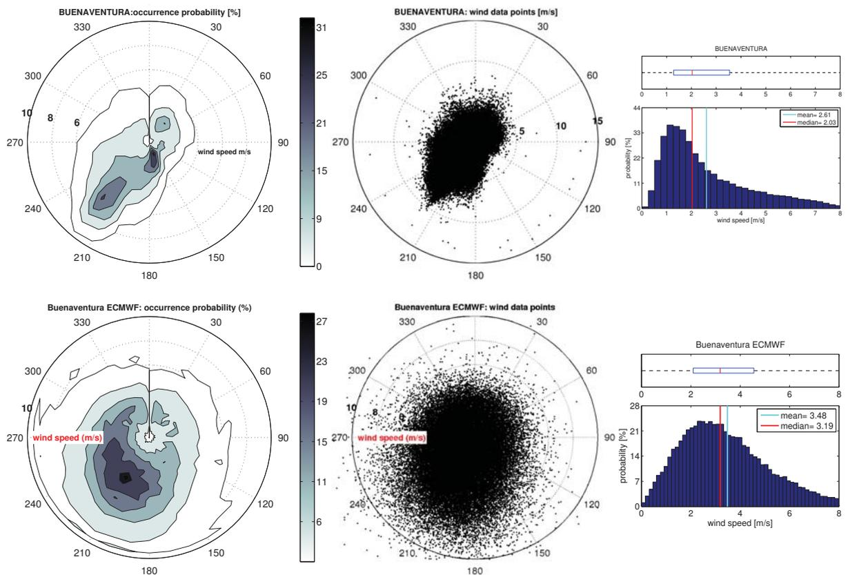
Figure 3: Wind statistics from observed records (upper panels), and from the ECMWF model (lower panels) at Buenaventura.
