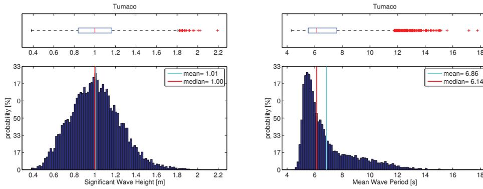
Figure 13: Statistics of integral parameters over the whole spectrum,  $H_{m0}$  (left) and  $T_{m-1,0}$  (right) at Tumaco.
